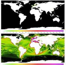
Geographical coverage in 2007 (top) and 2012 (bottom), coloured according to the intensity of satellite AIS messages received per unit area. This is a composite of both vessel activity and geographical coverage; intensity is not solely indicative of vessel activity (Corbett, Smith, Anderson 2014).
